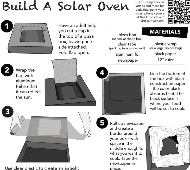
Use clear plastic to create an airtight window for solar energy to enter the box. Plastic wrap or a piece of a Ziplock bag
